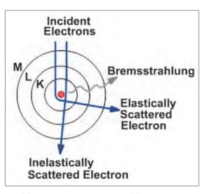
Figure 3. Scheme of X radiation or "braking radiation" (20)
