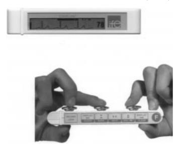
**Figure 2.** Small Tele-ECG monitoring device with metal contacts (Company IFE, Germany)
