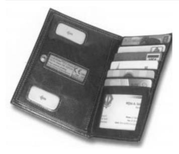
Figure 1. Wallet-like ECG recorder
